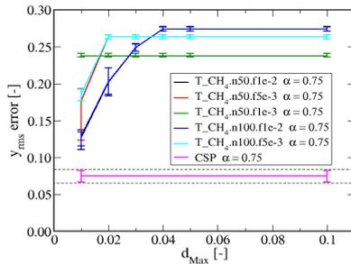
Fig. 3. Scaled RMS error in overall system state from CSP with and without tabulation compared to detailed chemistry simulations. The dashed lines indicate the errors for regular CSP. The errors are averaged over 100 simulations with randomly sampled initial conditions, with “error bars” indicating the 5% and 95% quantiles. Time step factor  $\alpha = 0.75$ .
