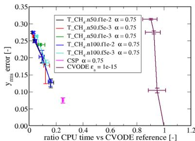
Fig. 4. RMS error versus relative CPU time for  $\text{CH}_4$ -air ignition simulated with detailed chemistry, or with CSP with and without tabulation. The reference is a detailed chemistry simulation with tight tolerances.
