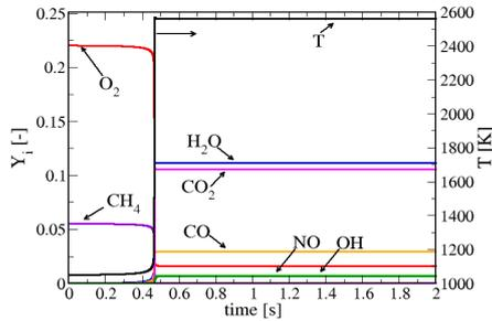
Fig. 1. Mass fractions of various species as well as temperature, in an igniting stoichiometric  $\text{CH}_4$ -air system.
